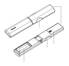
1.ON/OFF Button 2. "HOLD" Button 3.UV-C Bulb 4.Lithiumion Battery Box
